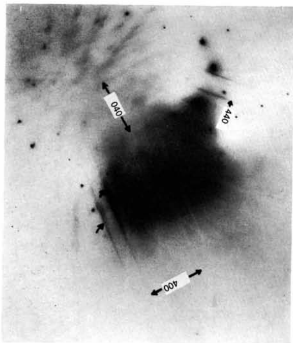
Fig. 3. Electron diffraction pattern of MgO crystal no. 3 (93 ppm Fe, slowly cooled from 1400°C).
